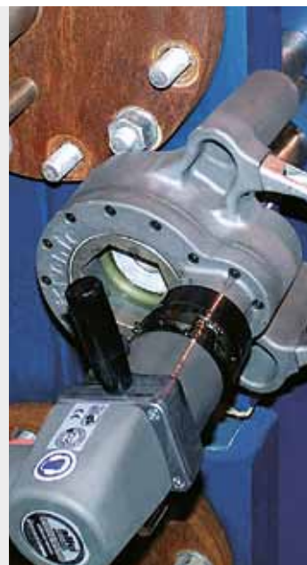
Image above: PWT of Alfa Laval Images on the right: alkitronic ® CLS-SG and RCL in operation on plate heat exchangers.
