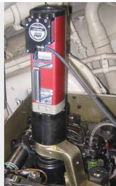
Applications alkitronic ® EFWip „all-weather“ design with protection class IP 54 (figure above) alkitronic ® EF , bolting application at a diesel engine (figure on the right)
